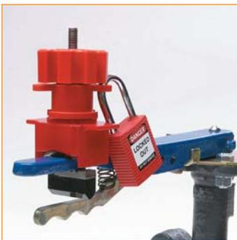
Clamp attaches to butterfly valve lever, preventing trigger handle from being squeezed. Valve cannot be repositioned!
